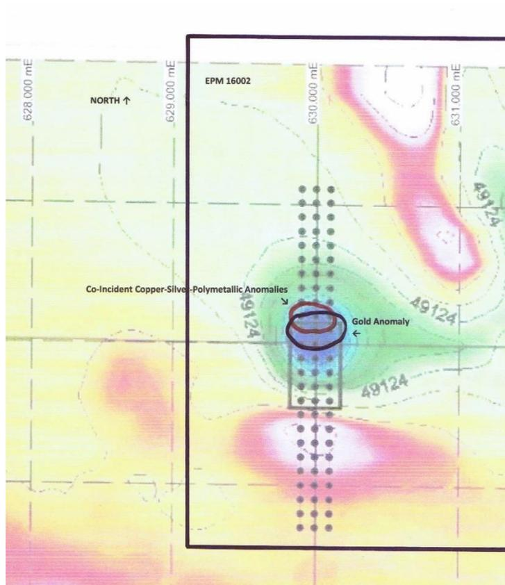
Figure 4: Co-incident Cu-Ag-Polymetallic SGH soil anomaly and partly overlapping Au anomaly draped over an aeromagnetic base.
