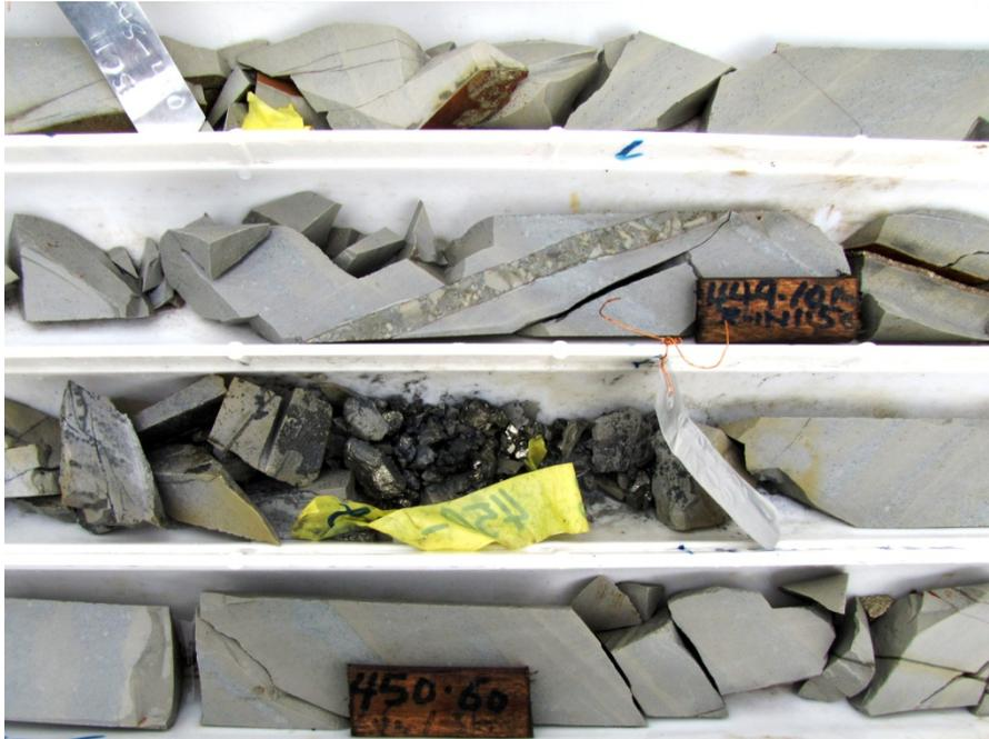
*NEV 018 showing part of sample interval 448m to 450m (2.0m at 1.64 g/t Au) with base metal sulphide - pyrite vein*
