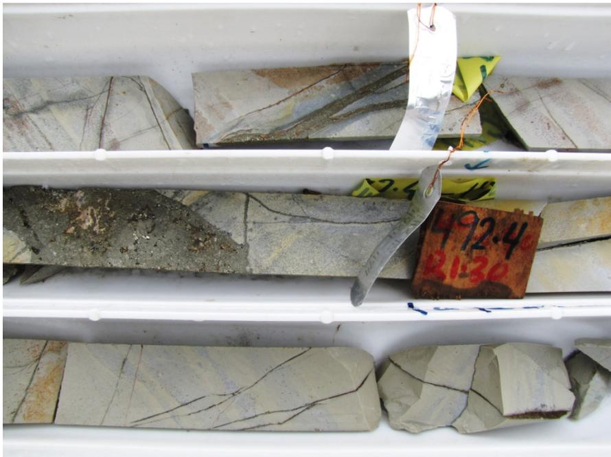
*NEV 018 showing part of sample interval 491.8m to 492.4m (0.6m at 1.57 g/t Au) with pyrite - minor base metal sulphide veins*
