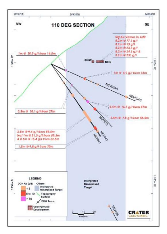
Figure 7 - Section of Drill Holes and Intercepts on 110° Bearing
