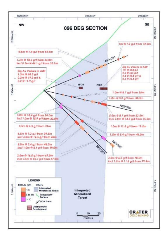
Figure 6 - Section of Drill Holes and Intercepts on 96° Bearing
