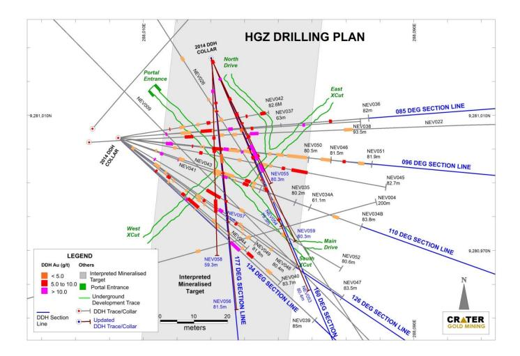
Figure 1 - Plan of Current Drill Hole Traces and Historic Drill Holes
