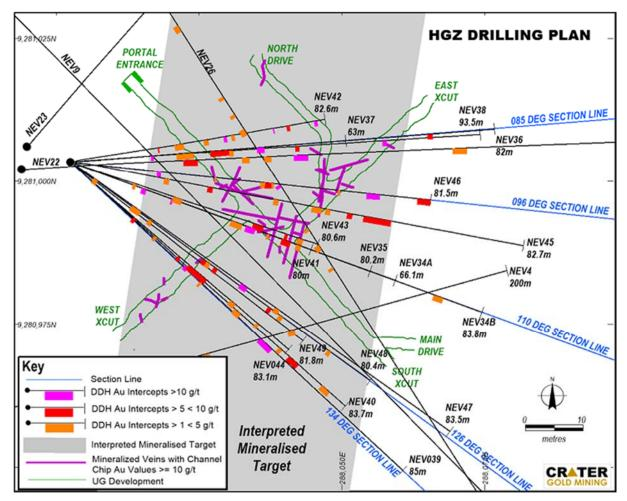
Figure 1 - Plan of Current Drill Hole Traces and Historic Drill Holes
