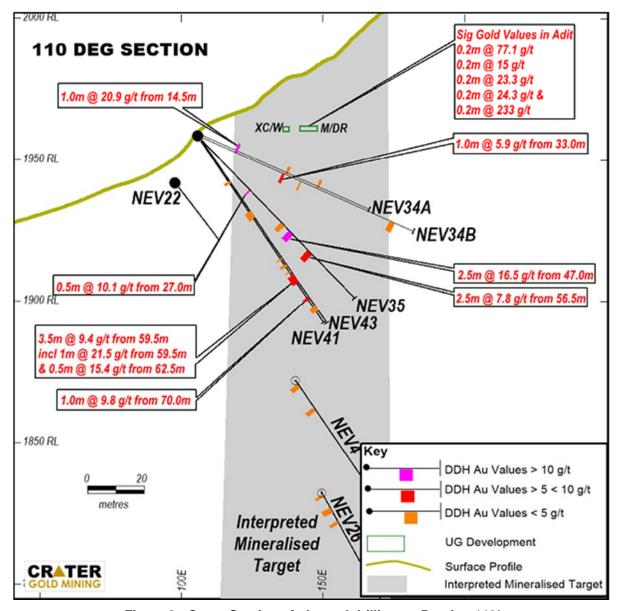
Figure 2 - Cross Section of planned drilling on Bearing 110°
