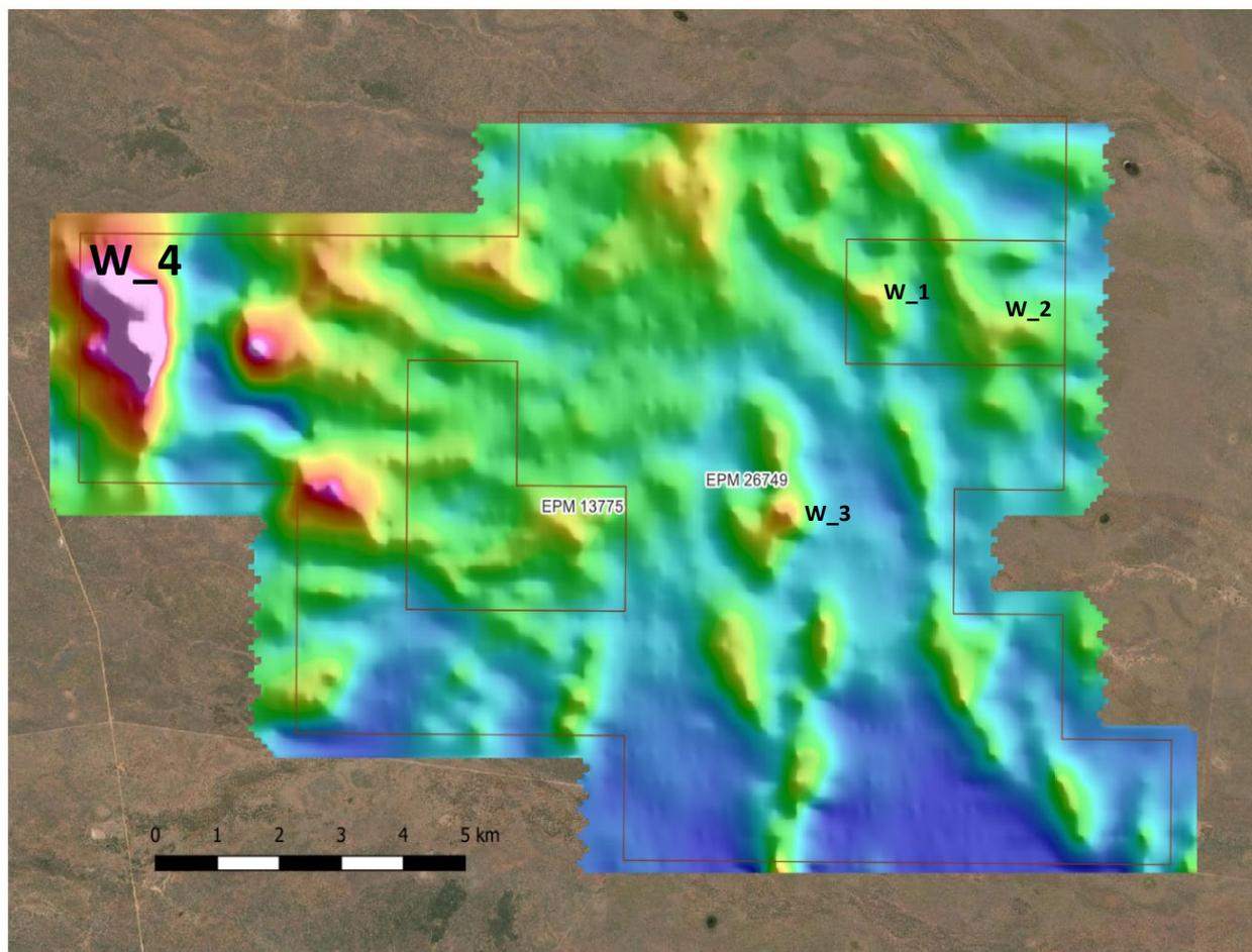
**Figure 6:** Image showing the large (W\_4) EM conductor in the NW corner of EPM 26749 and discrete low priority anomalies W\_1, W\_2 and W\_3. The WNW to N trending pattern of weak linear EM anomalies is related to cover, possibly reflecting faults or geological-trends in the bedrock.
