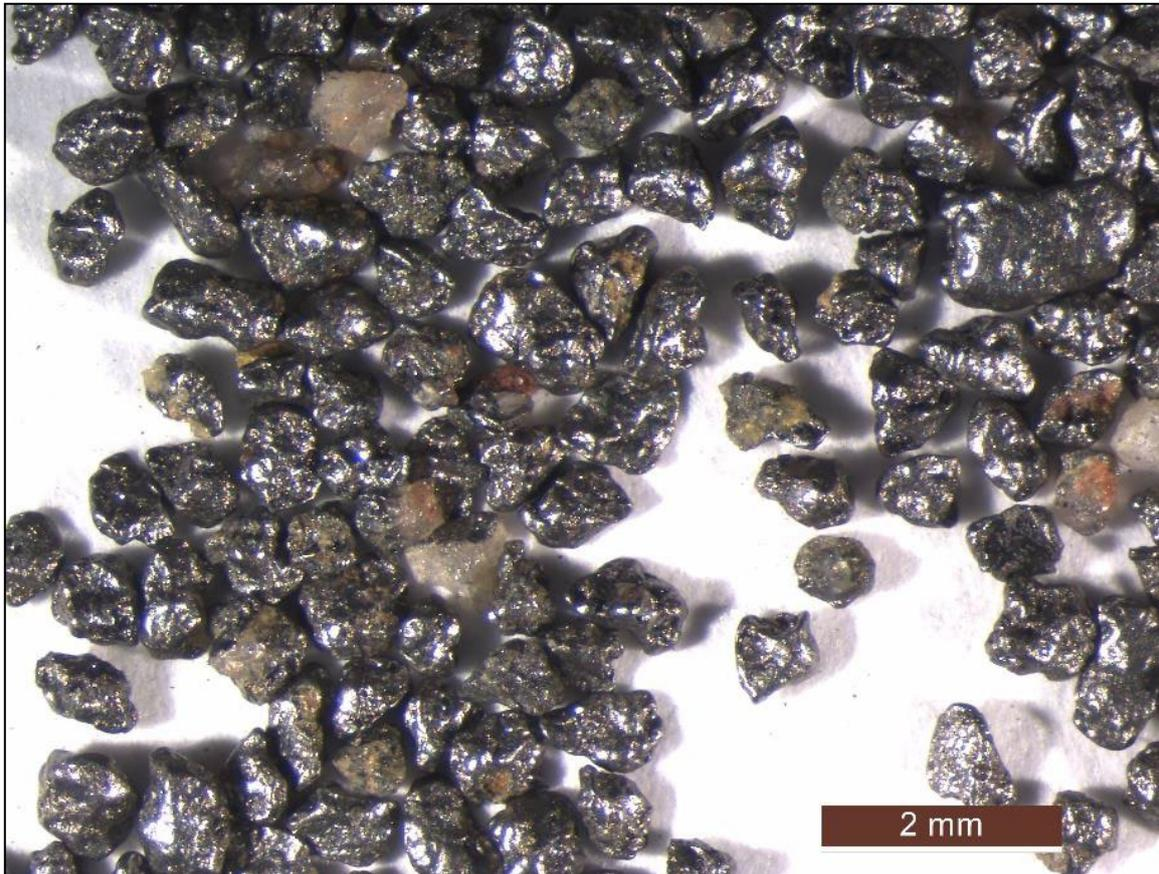
**Figure 2:** 1.0mm composite sample rougher concentrate, 500 microns fraction, showing sub-rounded graphite nodules and silicate gangue
