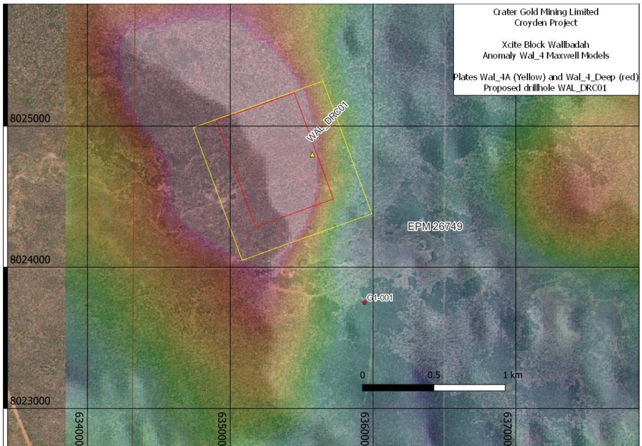
**Figure 7:** The large Anomaly W\_4 shown together with rectangular shaped blocks modelled from the data projected to surface. Drill hole WAL\_DRC01 has been selected to test this large anomaly. Previous unsuccessful hole G1-001, sited to test a residual gravity anomaly, lies some 1.2km to the SSE.
