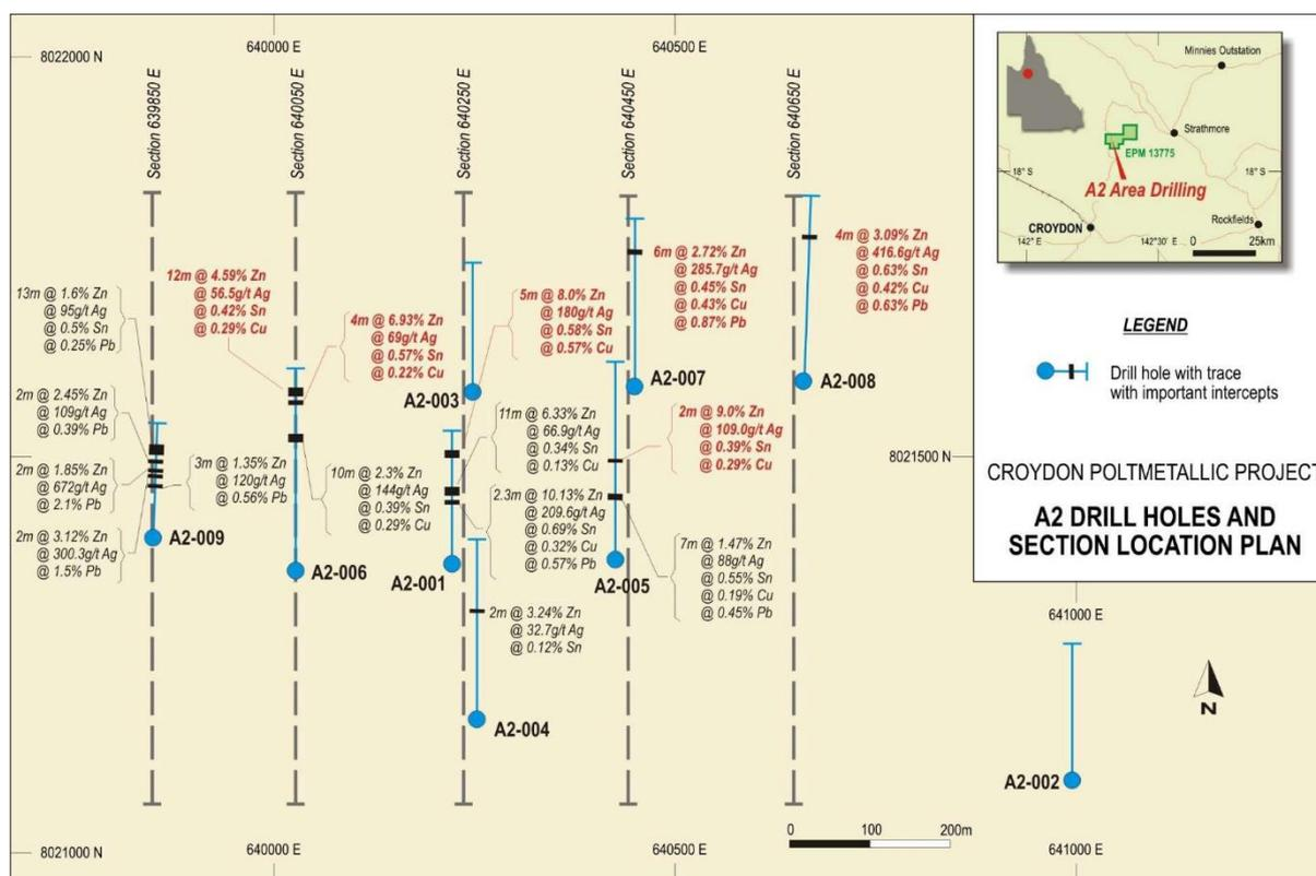
**Figure 3 (above):** Massive Sulphide Drill Hole Intersections at the A2 Anomaly.
