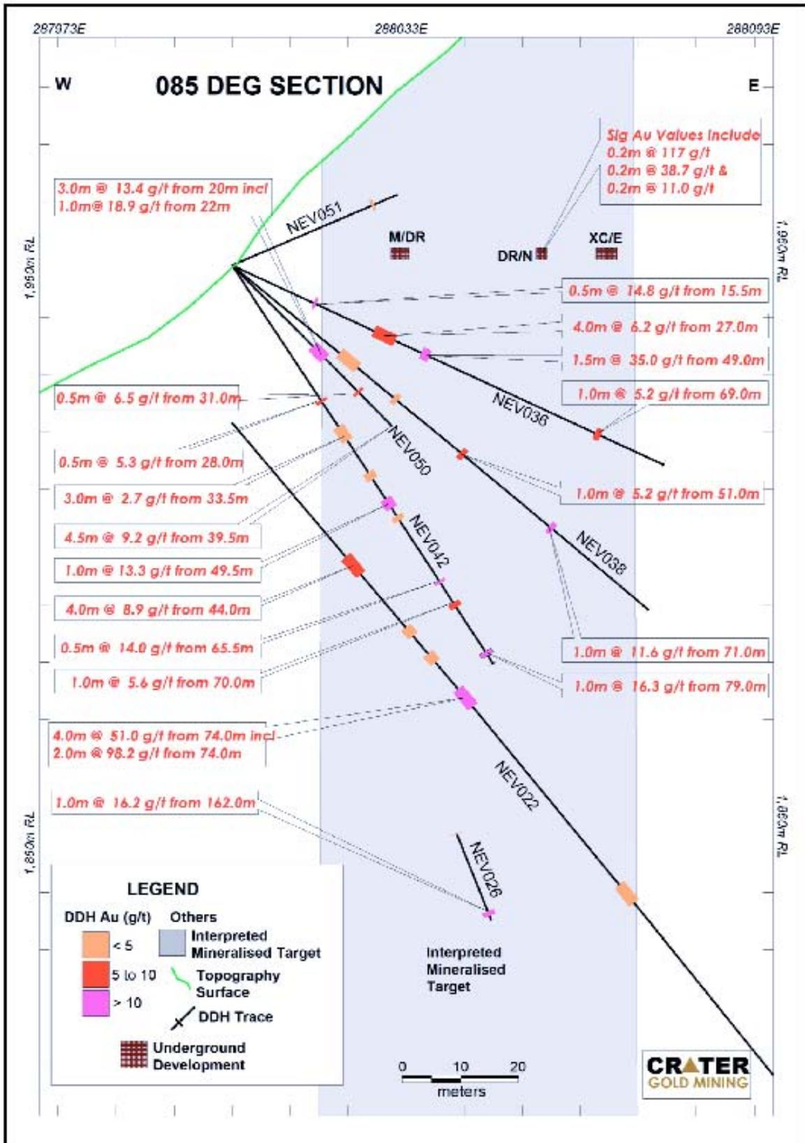
Figure 7 - Section of Drill Holes and Intercepts on 85° Bearing
