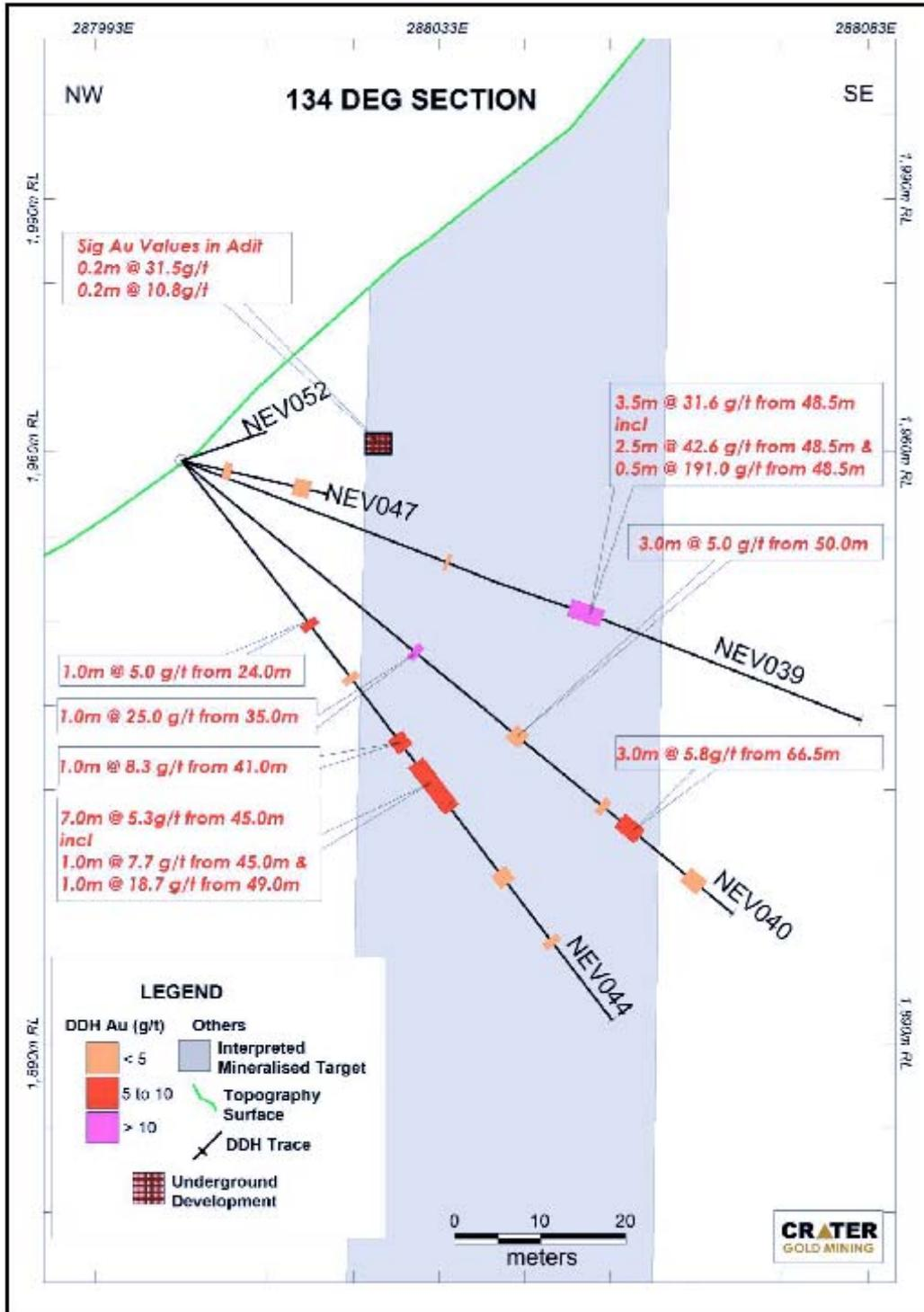
Figure 11 - Section of Drill Holes and Intercepts on 134° Bearing
