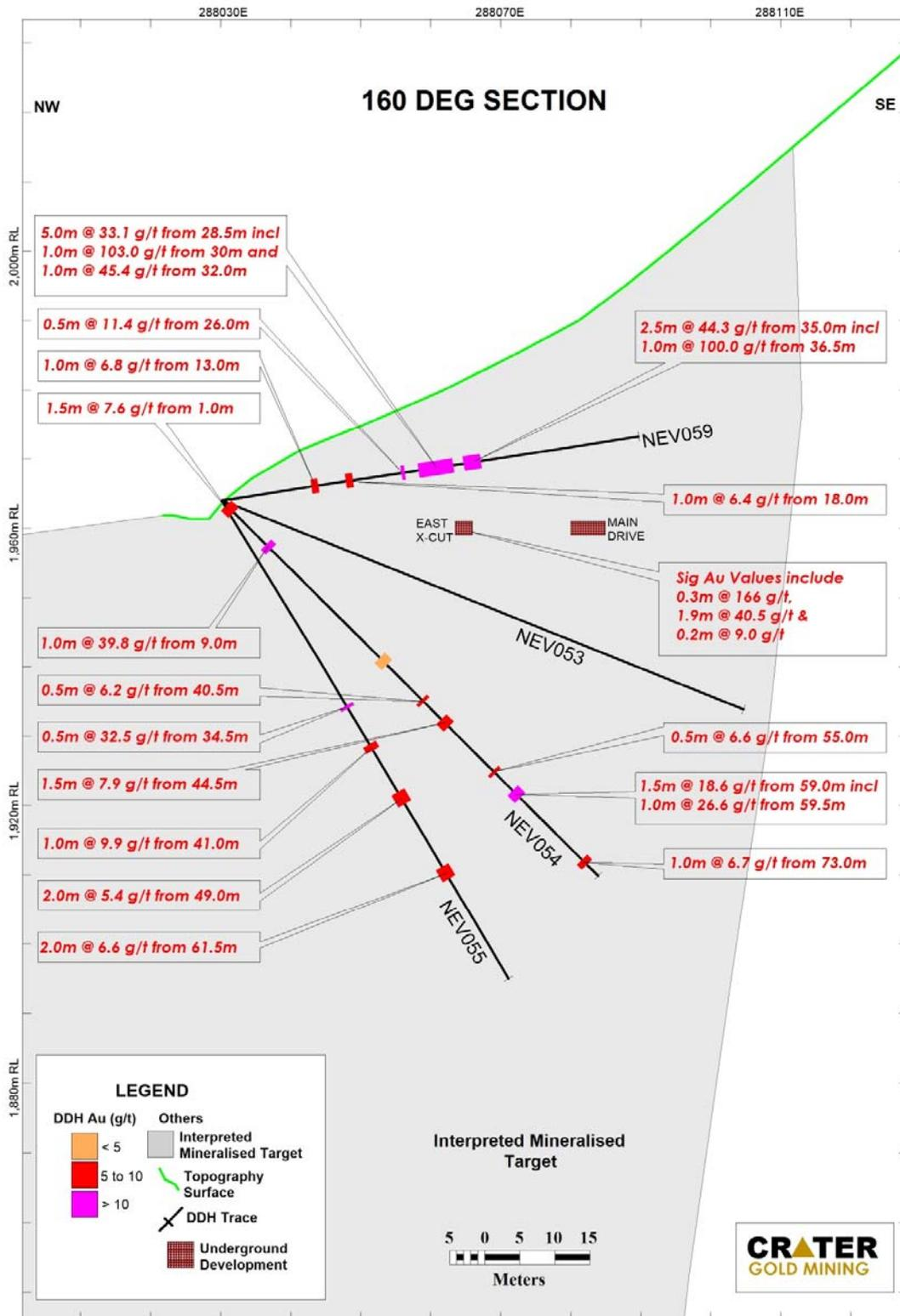
Figure 5 - Section of Drill Holes and Intercepts on 160° Bearing
