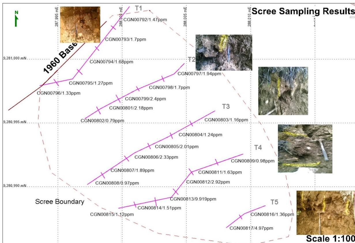
**FIGURE 2:** Scree Sample Trenches, Sample Numbers and Gold Assay Results (ppm)
