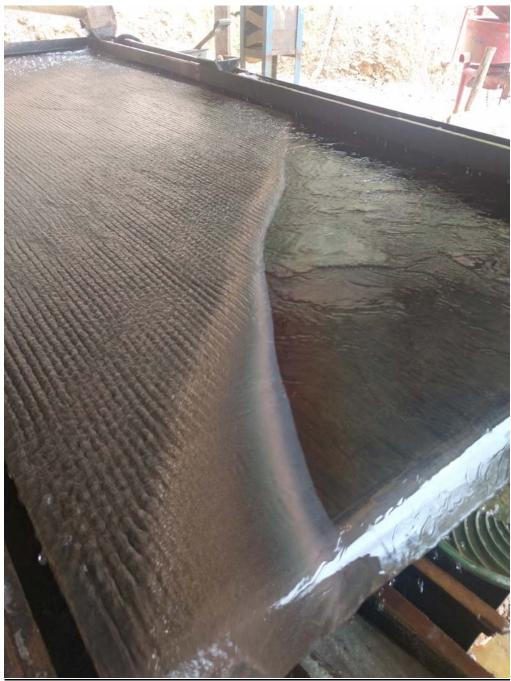
Figure 3 - Shaking table concentrate stream
