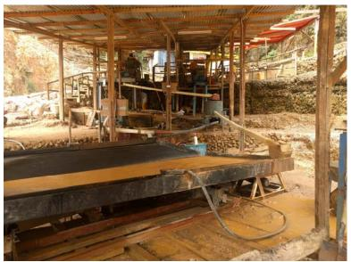
Figure 1 - Hammer mills, centrifugal concentrators and shaking tables
