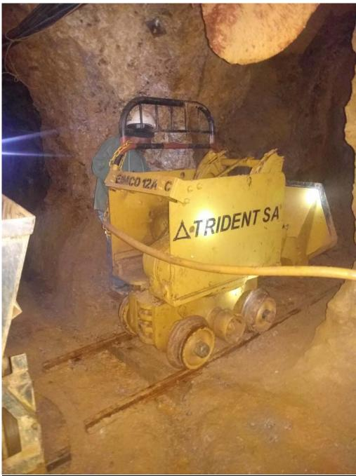
Figure 2 - Underground rocker shovel for mechanical loading
